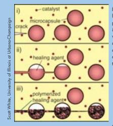
Left: The autonomic-healing concept. A microencapsulated healing agent is embedded in a structural composite matrix containing a catalyst capable of polymerizing the healing agent. i: Cracks form in the matrix wherever damage occurs; ii: the crack ruptures the microcapsules, releasing the healing agent into the crack plane through capillary action; iii: the healing agent contacts the catalyst, triggering polymerization that bonds the crack faces closed.
