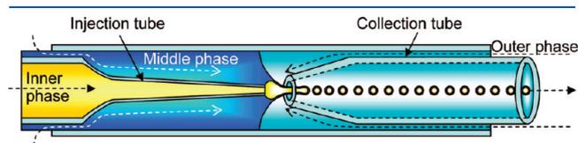
**Figure 3.** Schematic of a microcapillary device used for generating double emulsions.<sup>55</sup>
