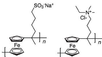
**Figure 6.** Ferrocene-containing polymers used for electrochemical triggering.<sup>65</sup>
