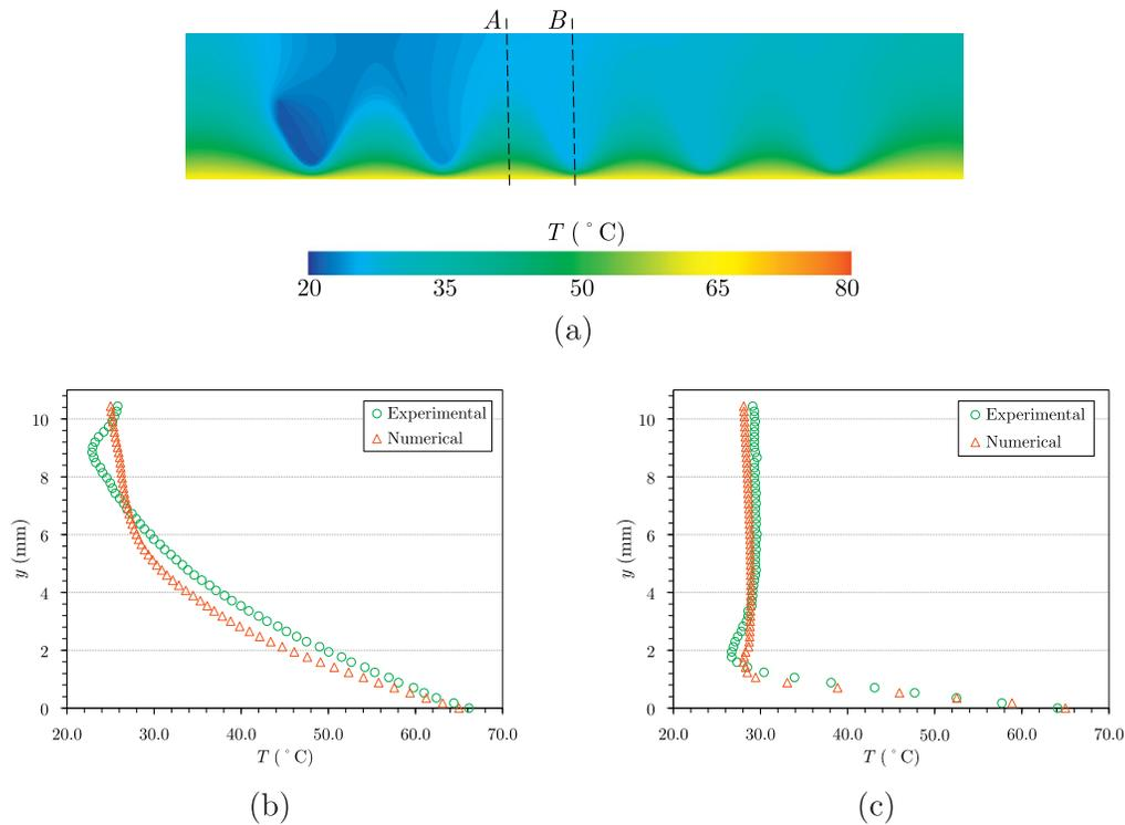
**Fig. 9.** Calibration of the IGFEM solver using the thermally loaded domain with an embedded microchannel with  $\lambda = 10$  mm: (a) steady-state temperature field of the actively-cooled fin at 2 ml/min flow rate obtained with the IGFEM; (b,c) experimental and numerical temperature profiles along Sections A and B, respectively.
