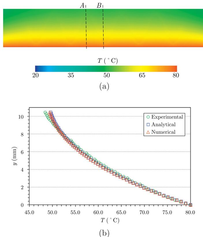
**Fig. 8.** (a) Temperature field obtained with the 2D IGFEM solver in the absence of the flow; (b) experimental, numerical and analytical temperature profiles along Section A. A heat transfer coefficient of  $h = 4.9 \text{ W/m}^2\text{K}$  is employed to evaluate the analytical and numerical solutions.
