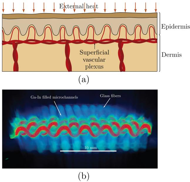
**Fig. 1.** Biological and biomimetic examples of microvascular systems for active cooling: (a) microvascular blood vessels for thermal regulation in the human skin (inspired from [13]); (b) micro-CT image of sinusoidal-shaped microchannels (filled with eutectic Ga–In alloy for a higher resolution) embedded in a 3D woven glass fiber/epoxy matrix composite created with the sacrificial fiber manufacturing technique.
