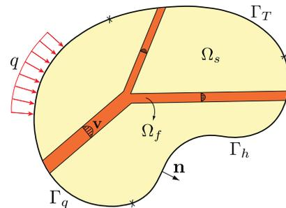
**Fig. 2.** Schematic of a 2D domain  $\Omega = \Omega_s \cup \Omega_f$  with the fluid ( $\Omega_f$ ) and solid ( $\Omega_s$ ) phases. The boundary  $\Gamma$  with outward unit normal  $\mathbf{n}$  is divided into regions  $\Gamma_T$ ,  $\Gamma_q$ , and  $\Gamma_h$  for assigning the Dirichlet, Neumann, and Robin boundary conditions, respectively.
