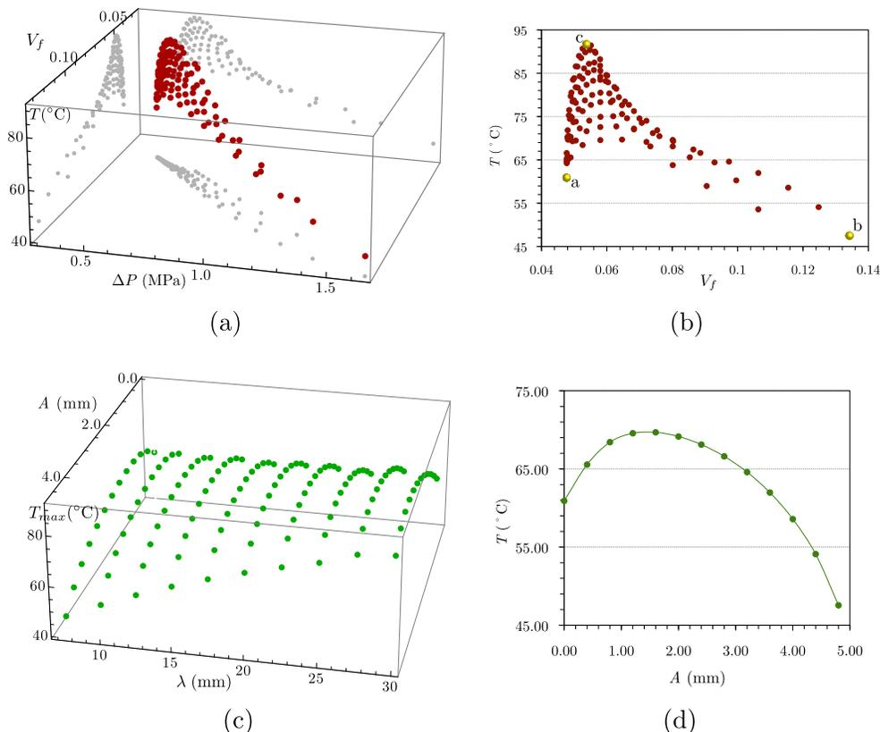
**Fig. 13.** Optimization results for the problem shown in Fig. 12 with a prescribed temperature along the top edge: (a) representation of three and (b) two objective functions for each individual; (c) maximum temperature versus the wavelength  $\lambda$  and microchannel amplitude  $A$ ; (d) maximum temperature in the fin versus the microchannel amplitude for  $\lambda = 7.5$  mm.
