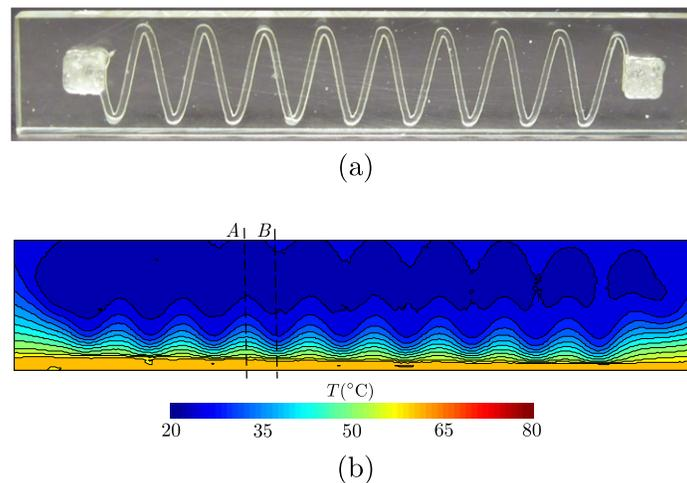
**Fig. 10.** (a) Microvascular fin specimen with an embedded microchannel with wavelength  $\lambda = 5$  mm and amplitude  $A = 4$  mm; (b) IR image of the steady-state temperature field after active cooling at 2 ml/min flow rate.
