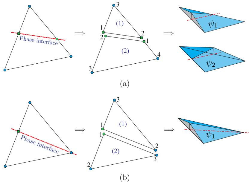
**Fig. 4.** Evaluating the enrichment functions in the IGFEM. Figs. (a) and (b) illustrate two scenarios for creating integration elements and the associated generalized dofs for three-node triangular elements based on the location of the phase interface.
