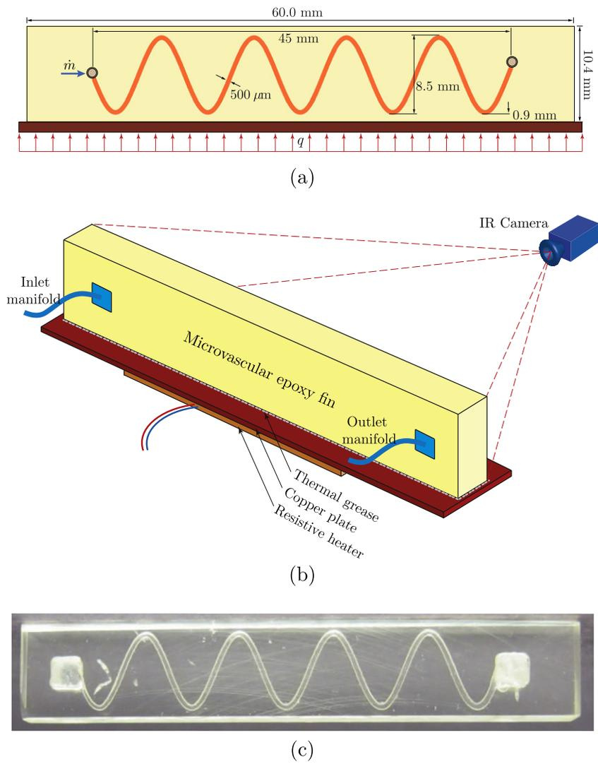
**Fig. 6.** (a) Geometry and boundary conditions of the validation study performed on a thermally loaded microvascular epoxy fin with a 500  $\mu\text{m}$  diameter sinusoidal embedded microchannel; (b) schematic of the experimental set-up with infrared imaging of the temperature field on the surface of the fin; (c) microvascular epoxy fin specimen with embedded microvascular channel created by the direct ink writing technique.
