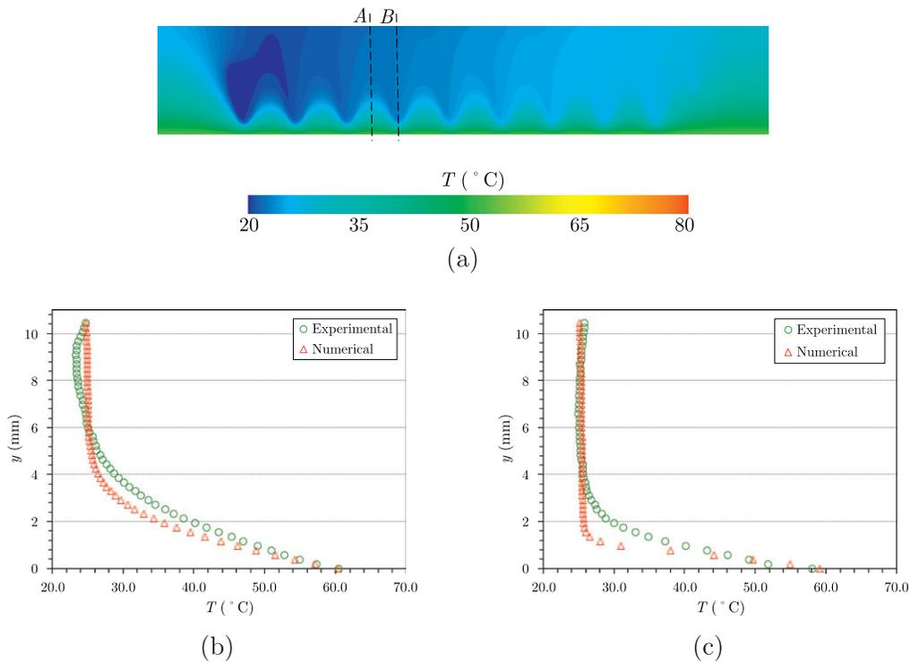
**Fig. 11.** Validation of the IGFEM solver based on the microvascular fin with  $\lambda = 5$  mm: (a) steady-state temperature field of the actively-cooled fin at 2 ml/min flow rate obtained with the IGFEM; (b,c) experimental and numerical temperature profiles along Sections A and B, respectively.
